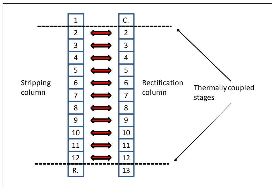
**Fig. 4.** Numbering of the plates and equilibrium stages in HIDiC
