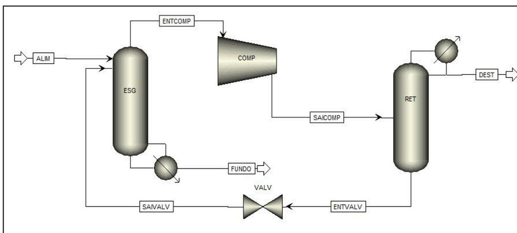
**Fig. 1** – Illustration of a HIDiC column in Aspen software
